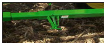
Snap Pin used When Switching Between Transport and Articulation Mode
