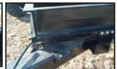
UHMW Wear Plate on Rear Axle
